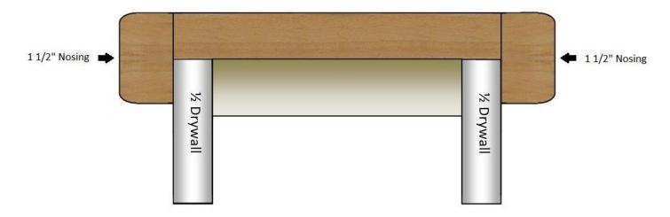
If the R2E trim is too slim for your liking, you can also use a standard 1 1/2" nosing. The cap piece is the same width as the wall and the nosing is fitted flush with the top. This creates the illusion of a thick cap, and easily hides the drywall seam.
