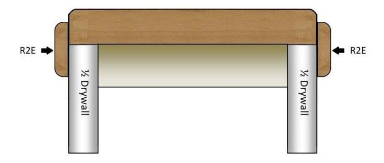
For a sleeker finish a cap piece the same width as the wall is fitted to match the edge of the drywall. Our slim trim, the R2E is used to cover the seam between the drywall and the cap. The drywall cut does need to be a little more precise as there is less trim to cover the seam. Custom trim can always be made if you need something specific to finish your project.
