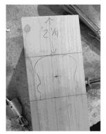
1. On your post, mark where you want the final position of your rail to be. In this example, it will be 2 1/4" from the top of the post. Also, mark the centre point of the rail outline. This will be where your rail bolt connects to the rail once it's anchored to the post
