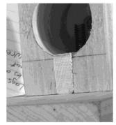
Using a 1/2" piece of fillet, or some other material, make a tapered wedge to glue into this slot, and glue your plug after as described above
