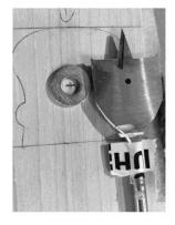
Tip: Mark with tape on a 1 1/2" spade bit, the depth allowed for the bit to be drilled from the bottom of the rail. When you go to drill the rail from the bottom, you want to have enough depth to allow the rail bolt's washer to sit properly, but not to drill too deep so as to poke the top of the rail
