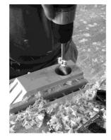
6. Begin to drill your 1 1/2" hole on the bottom of your rail down to your tape marker. Ensure the drill bit is drilling as straight as possible with minimal lateral vibration
